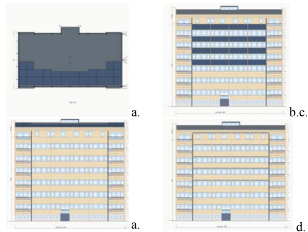
Fig. 4: Analyzed design variants: a. I Design Variant: roof 40° (roof and facade layouts), b. II Design Variant: parapet 90°, c. III Design Variant: parapet 45°, d. IV Design Variant: sun shading 0°
